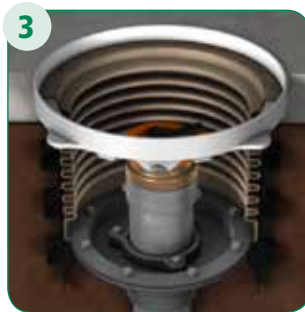
3 Replace Bellows, Reinstall Upper and Lower Rings
