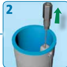
Lift float with cable to simulate fill
