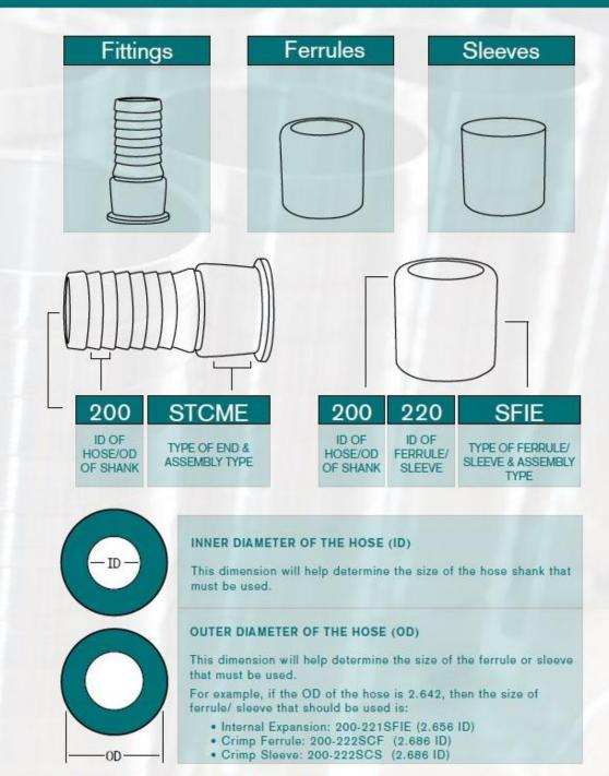
Quick Note: When the OD of the hose is determined, match it with the closest ID of a ferrule.
