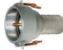
Aluminum Vapor Recovery Coupler with Probe Female Coupler Poppet with Viton Seal x Hose Shank
