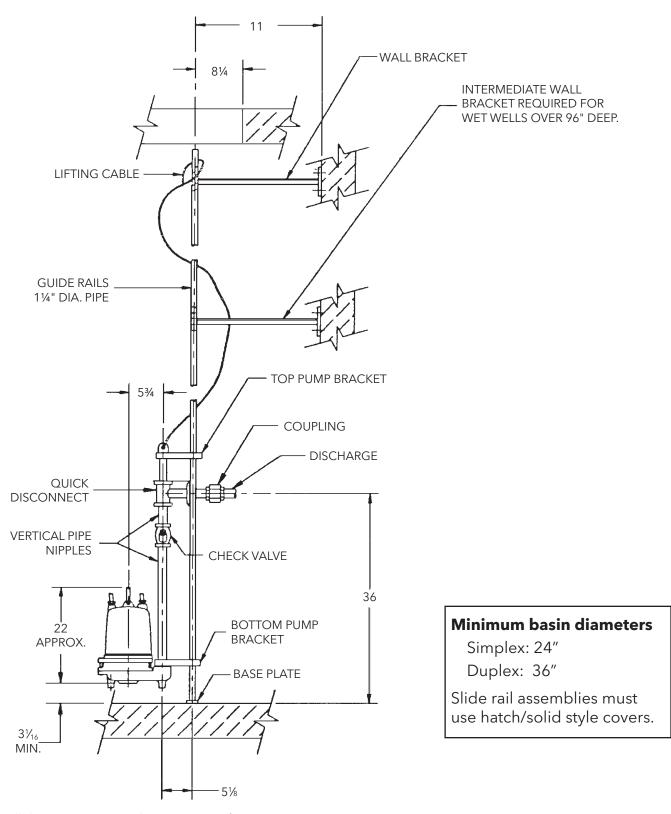
(All dimensions are in inches. Do not use for construction purposes.) \*\*To use catalog  $1\frac{1}{4}$ " Duplex Discharge Piping.
