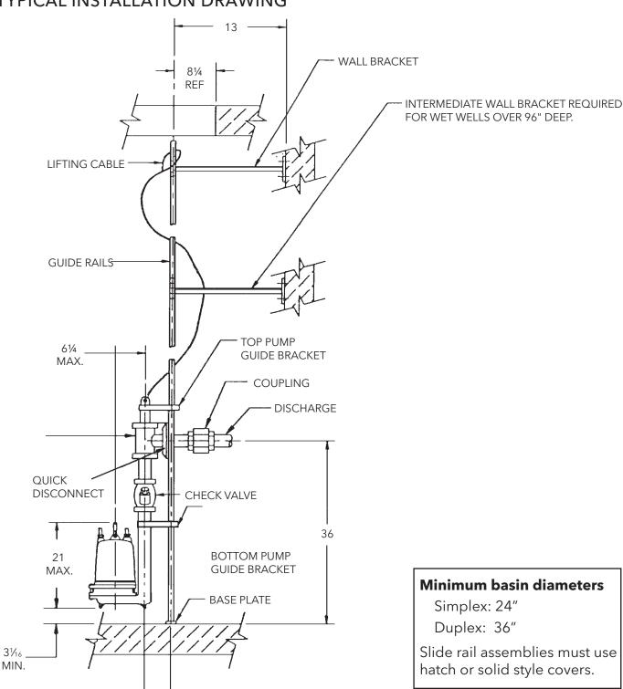
Slide rail assemblies must use hatch or solid style covers.
