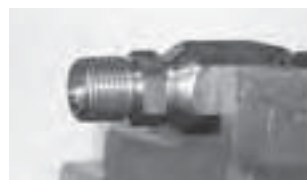
Stem properly seated against socket.
