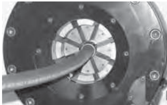
Insert hose assembly into crimper die set.
