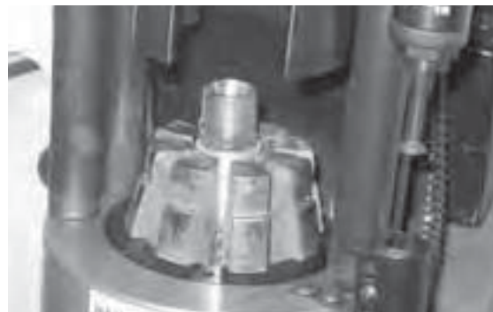
Insert hose assembly into crimper die set.
