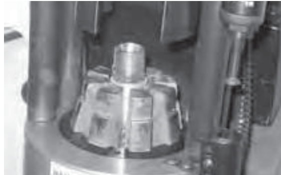
Insert hose assembly into crimper die set.
