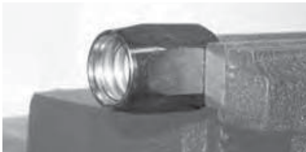
Socket positioned in vice.
