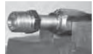
Screw stem into socket.
