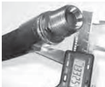
Verify crimp diameter with calipers.
