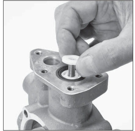
6.12 Install inlet valve (20) with flat side down onto plunger (21).
