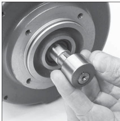
5.5 Remove and inspect cam (8) from motor shaft.
