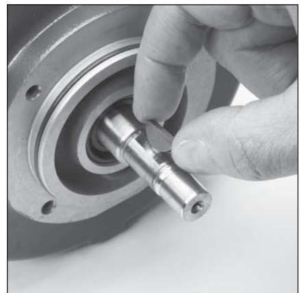
5.6 Remove and inspect woodruff key (9) from keyway of motor shaft.
