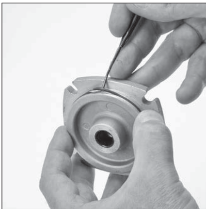
6.7 Lubricate and install o-ring (6) onto bearing cover (5).
