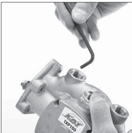
5.10 Insert the short end of an allen wrench to remove discharge valve assembly.
