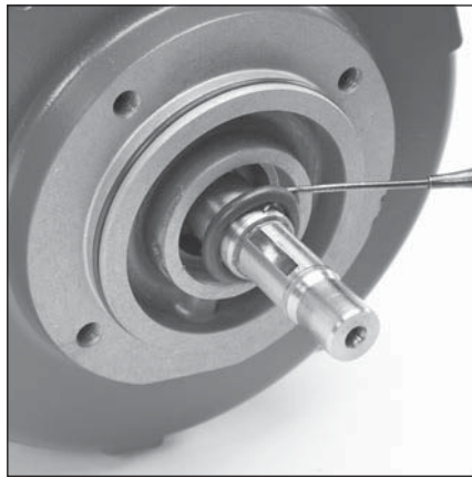
5.8 Use a pick tool to remove slinger o-ring (11) from motor flange.
