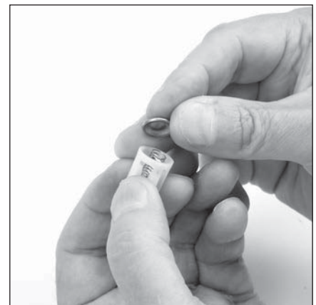
6.18 Place valve (25) cupped side over the spring (26).
