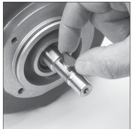
5.6 Remove and inspect woodruff key (9) from keyway of motor shaft.
