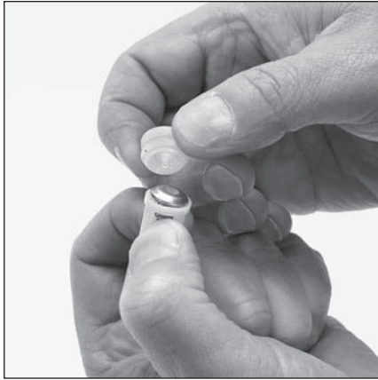
6.19 Place tapered side of seat (24) towards retainer (27) and snap into place.
