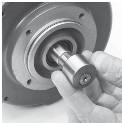
5.5 Remove and inspect cam (8) from motor shaft.
