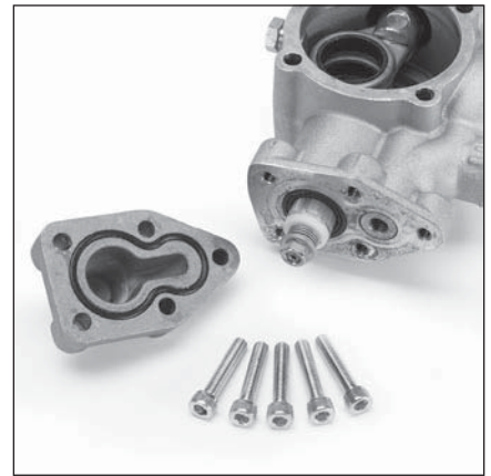
5.9 Use a 5mm allen wrench to remove five (5) M6x30 screws (13) holding head cover (14) to crankcase body.
