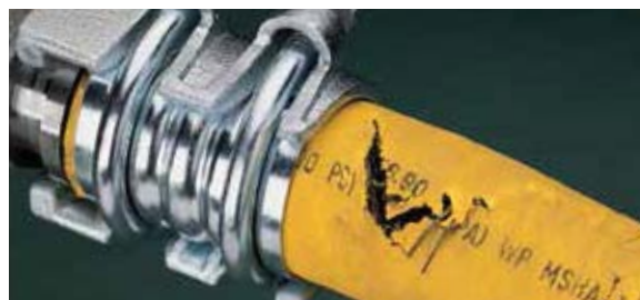
This 2" 1000 psi rated hose exploded in a test at 5200 psi. The hose exceeded its minimum 4X safety factor. The fitting and clamp exceeded the capacity of the hose.
